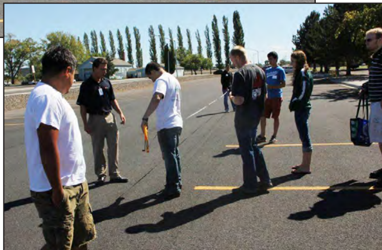
Scott Bernhardt, Takata Program Manager, explains the skid test to students at the STEM Summer Institute (above). After the test is conducted (above right), students measure the skid marks (right) and use the information to calculate how fast the car was going.
